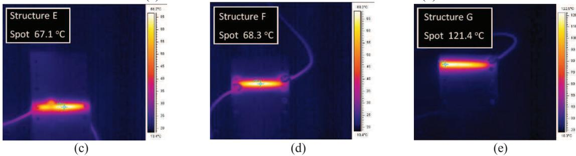
Fig. 4. I-T characteristics for traces E-G (Fig. 1) with 18  $\mu\text{m}$  (a), 35  $\mu\text{m}$  (b) layer thickness ; IR images of traces with the mentioned structures for 7.5A current and 18  $\mu\text{m}$  thickness (c) –(e).
