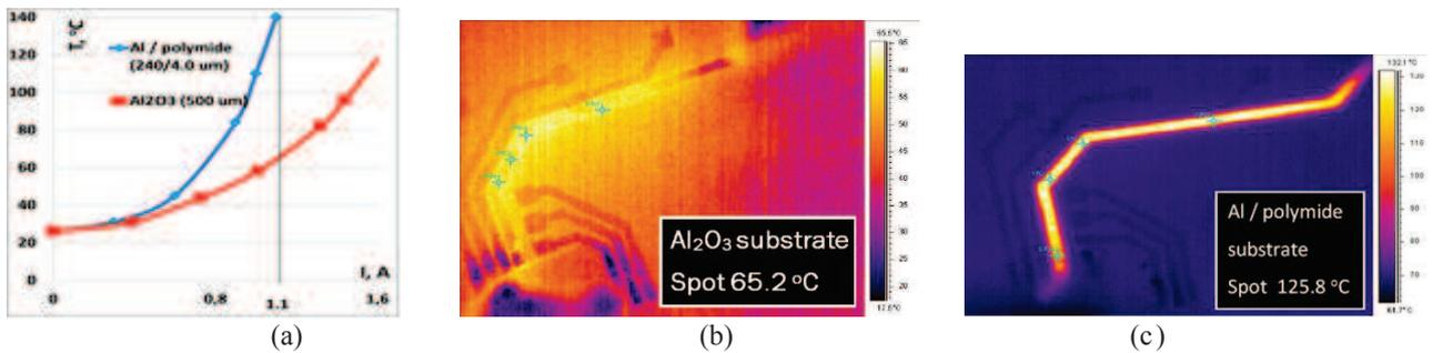
Fig.6. I-T characteristics (a) for high density traces (Fig 2) for different substrates; IR trace images (for current of 1.1A) for trace placed on a ceramic (b) and Al/polyimide (c) substrates .
