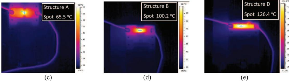
Fig. 3. I-T characteristics for traces A-D (Fig. 1) with 18  $\mu\text{m}$  (a), 35  $\mu\text{m}$  (b) layer thickness. IR images of the mentioned traces for 7.5A current and 18  $\mu\text{m}$  thickness (c) –(e).
