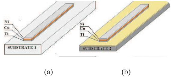
Fig. 2 Structures of modern high density test board: with ceramic  $\text{Al}_2\text{O}_3$  (500  $\mu\text{m}$ ) substrate (a), with aluminium / polymide (240 / 4,0  $\mu\text{m}$ ) substrate (b).
